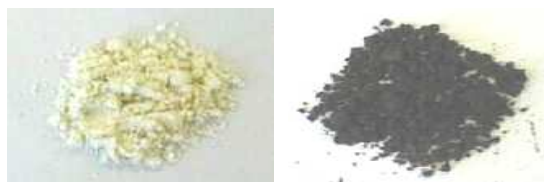
Figure 7. Crude products produced by Pd/C (left) and by Pd(OAc) 2 (right)
